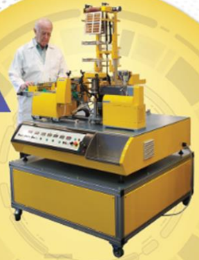
THE COMBI FILM BLOWING AND CHILL ROLL LINE WITH ONE COMMON EXTRUDER
